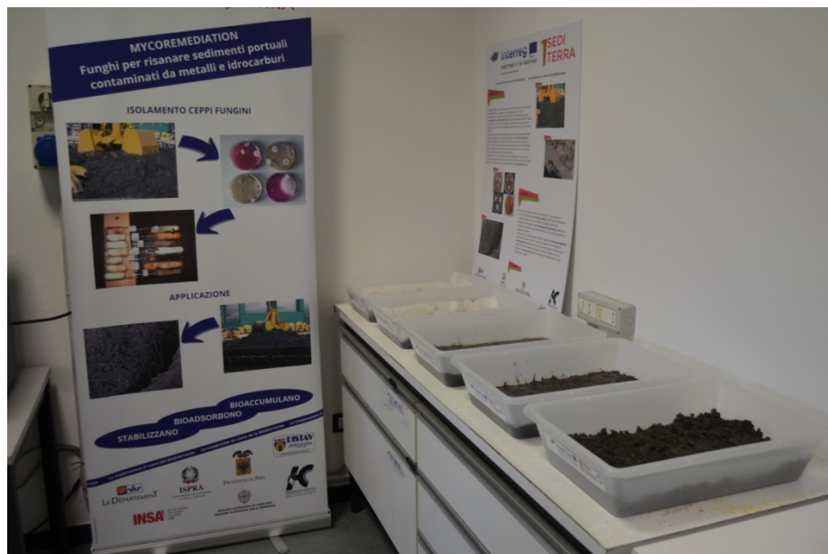
Figure 1. The five mesocosms used for the pilot activities: the two boxes on the left side are equipped with the membranes while the first one on the right of the photo is the C (control) box.
