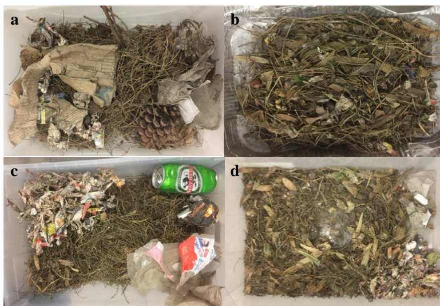
Fig. 3 Material composition analysis of: (a) d > 76.2 mm (sample 1); (b) 12.7 < d < 25.4 mm (sample 1); (c) d > 76.2 mm (sample 2); (d) 12.7 < d < 25.4 mm (sample 2).
