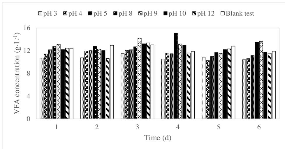
**Figure 6:** Effect of pH on VFA production in batch
