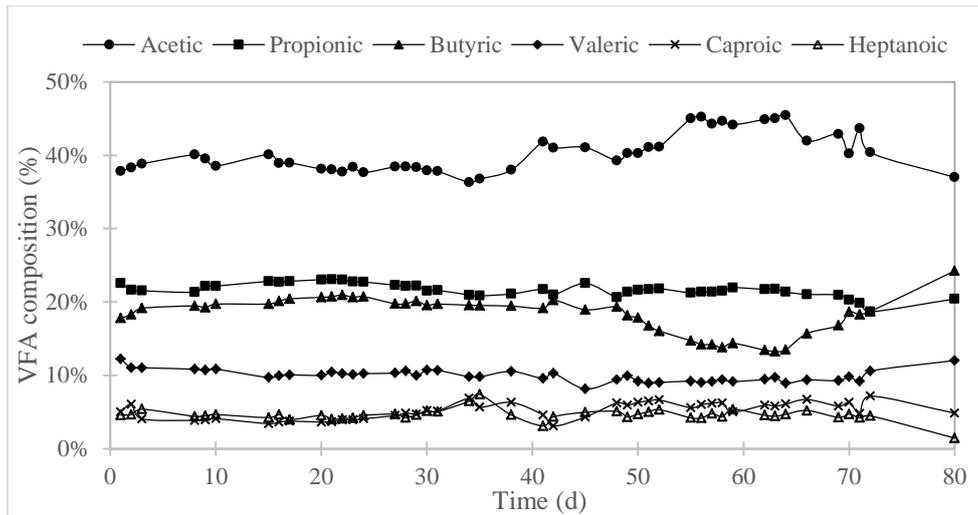
**Figure 5:** Selected particular VFA production under hyperthermophilic conditions (70 °C)
