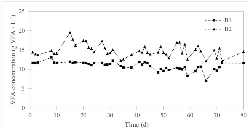
**Figure 2:** Effect of temperature on VFA production at 35 °C and 70 °C
