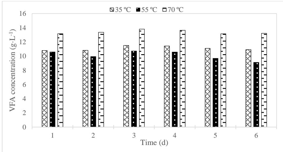
**Figure 1:** Effect of temperature on the evolution of VFA in batch at 35°C, 55 °C and 70 °C
