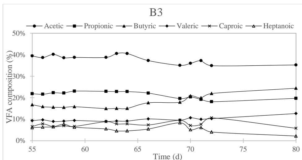
Figure 7: VFA composition at pH 10 and hyperthermophilic temperature
