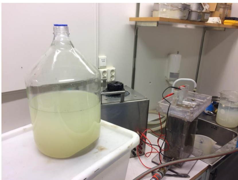
Figure 8. Gas wastewater mixed with zeolites and EC power source and reaction chamber.
