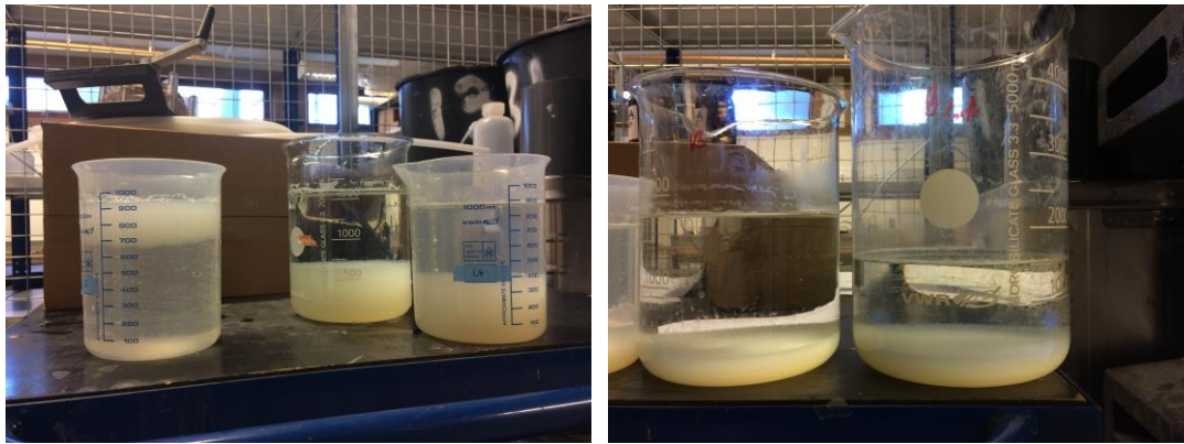
Figure 9. After EC from left: gas wastewater, mixed with 10 g and 100 g zeolites, and 100 g zeolites after 24 hours settling.
