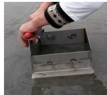
Figure 2: Newly developed excavation device for microplastic sediment sampling
