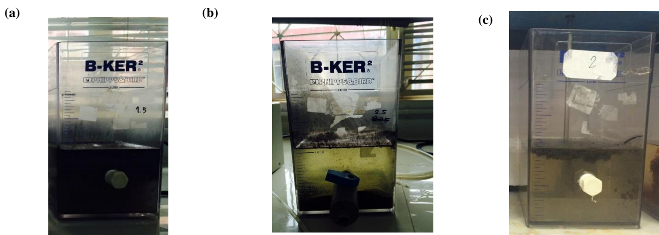
Fig. 1 (a) Initial MWF wastewater, MWF wastewater after (a) coagulation with \text{FeCl}_3 at 2.25 g/L (b) without polymer and (c) with 0.2 g/L of anionic polymer.
