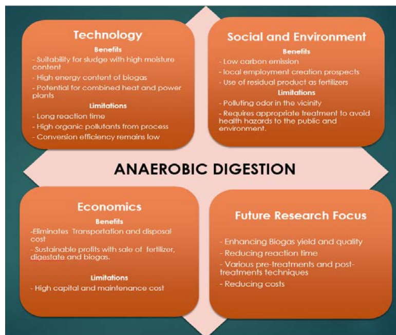
Figure 2: Technological, socio-environmental and economical assessment of anaerobic digestion for sewage processing
