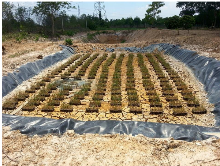
Figure 1 (a) Illegal dumping of TPH contaminated wastewater, (b) treatment of TPH contaminated water by vetiver on floating platforms in HDPE pond 1, and (c) treatment of TPH contaminated sediment by vetiver on landfarming in HDPE pond 2.
