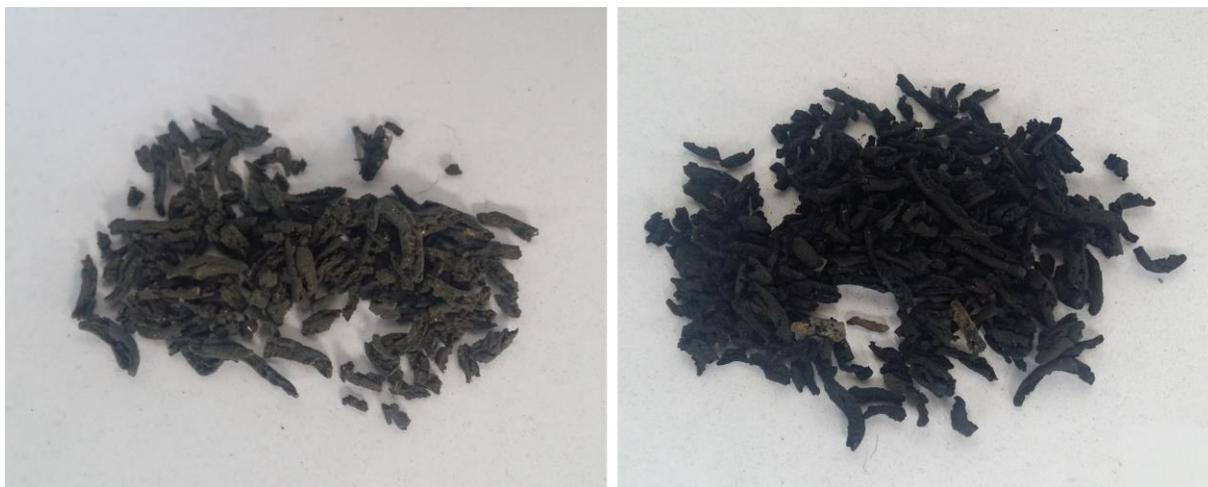
Figure 1. SS (SS2) before MP with noodle shape (left), biochar (BC2) after MP (right).
