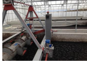
Picture 4. Solar drying system – mechanical mixing rotation drum
