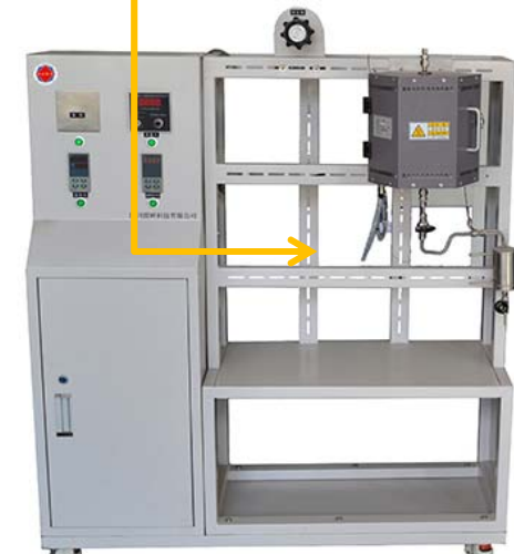
Fixed bed adsorption reactor
