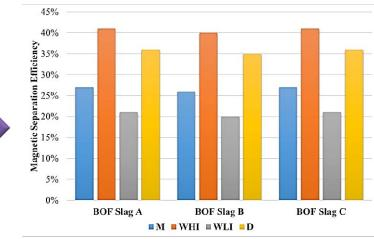
Wet High Intensity Magnetic Separation appears the best tecnique in terms of efficiency to be used for the separation of the magnetic matter from all the three tested BOF slags
