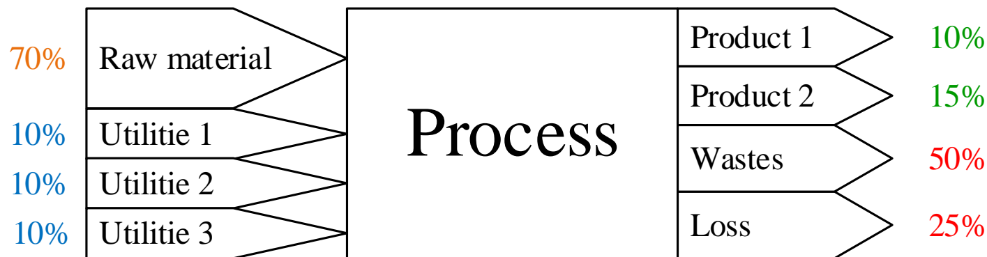
Figure 3. Main items involve in the energy distribution of the process
