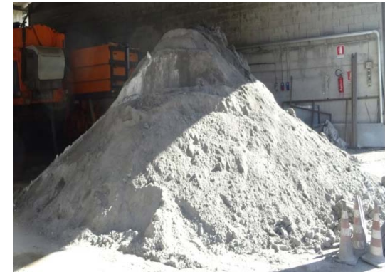
Dried aggregate sludge
