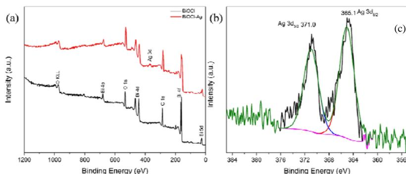
**Figure 4.** Survey spectrum of BiOCl and BiOCl-Ag (a); high resolution Ag 3d band (b).
