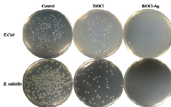
**Figure 6.** Photos of bacterial colonies formed by *E. coli* and *B. subtilis* cells treated by BiOCl and BiOCl-Ag after 2 h irradiation (concentration of catalysts:  $1\text{ g L}^{-1}$ ).
