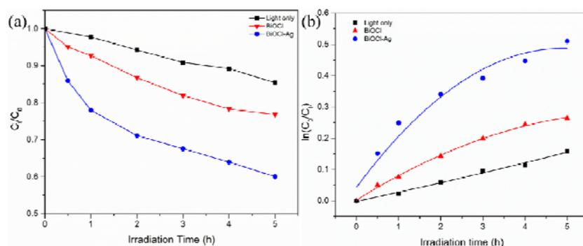
**Figure 5** Degradation rate of SNM by light, BiOCl and BiOCl-Ag (a); Kinetic plot of degradation of SAM (b); (concentration of catalysts:  $1\text{ g L}^{-1}$ )
