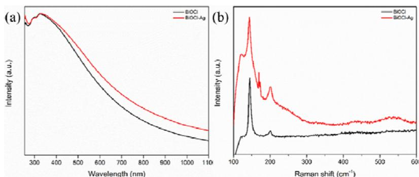
**Figure 3.** Comparison of UV-vis spectra of BiOCl and BiOCl-Ag (a); Comparison of Raman spectra of BiOCl and BiOCl-Ag (b).
