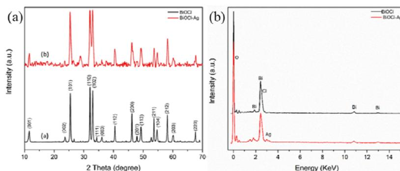
**Figure 2.** XRD patterns (a) and EDX (b) of BiOCl and BiOCl-Ag composites.
