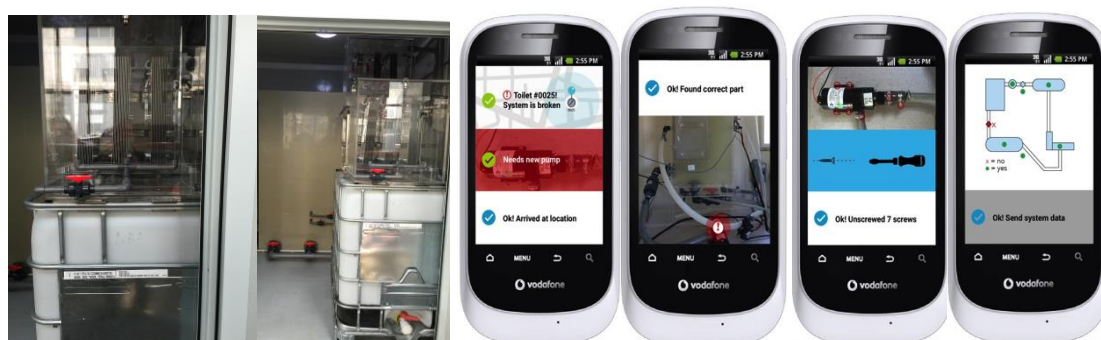
Figure 2 Left Panel: Alpha prototype showing the electrochemical reactor arrays, the baffled anaerobic reactor, flushwater tank, and the biochemical reactor effluent holding tank. Right: Smartphone monitoring and control systems for operational control, maintenance, and repair directions.
