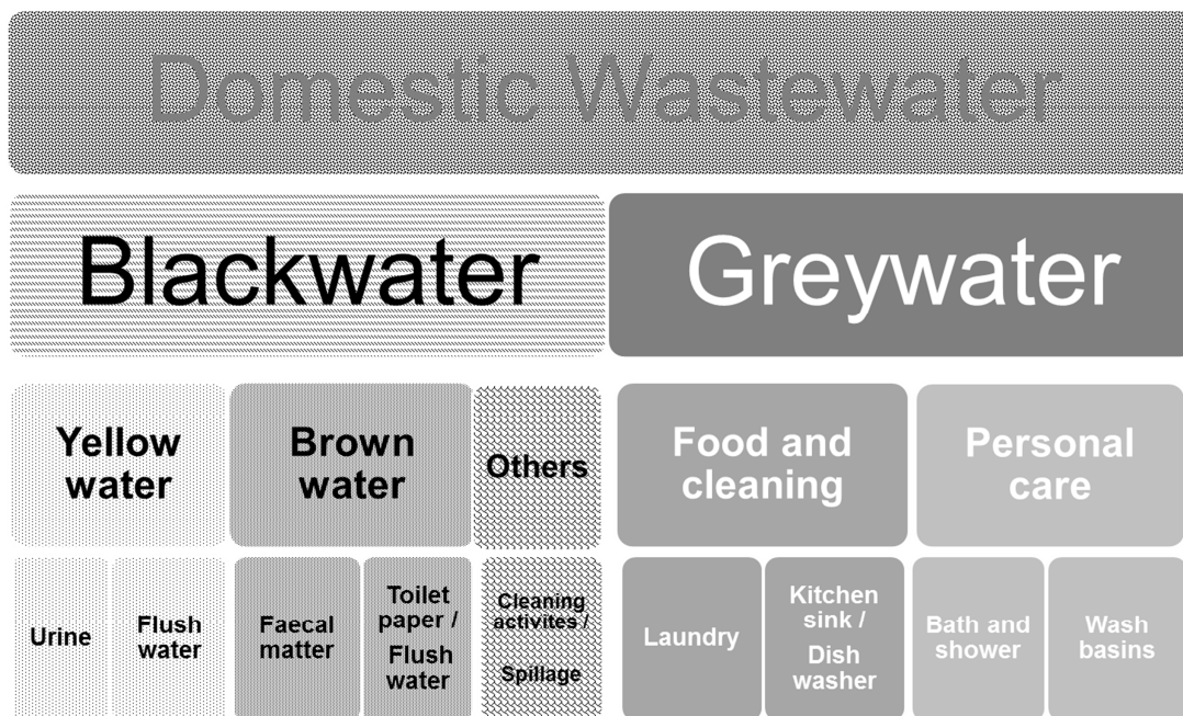
Figure 1. Classification of domestic wastewater
