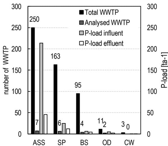
**Figure 2.** Overview of the treatment technology of WWTP in MV with less than 10'000 PE from the year 2014
