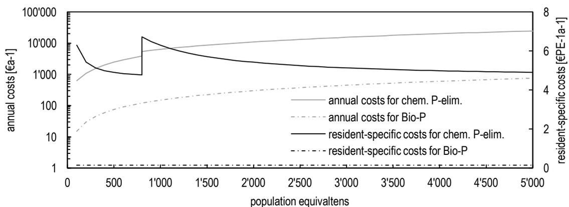
**Figure 11.** Comparison of the costs of biological and chemical methods, conditions: disposal costs: 300 €t<sup>-1</sup> excess sludge
