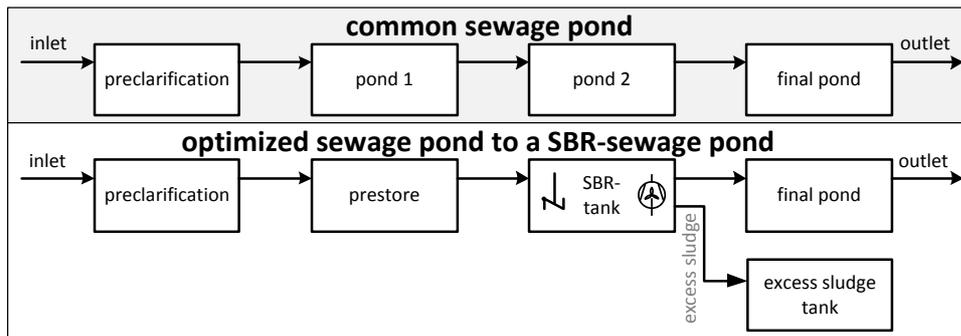
**Figure 8.** Schematic treatment technology of sewage ponds
