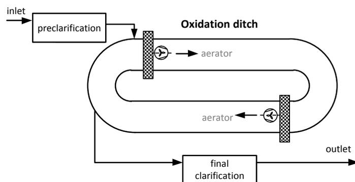
**Figure 10.** Schematic of the treatment technology of an oxidation ditch
