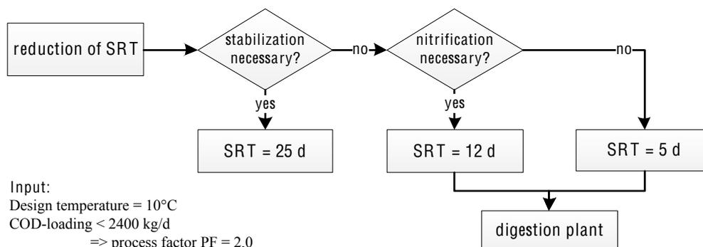
**Figure 6.** Determination of the minimum possible sludge retention time
