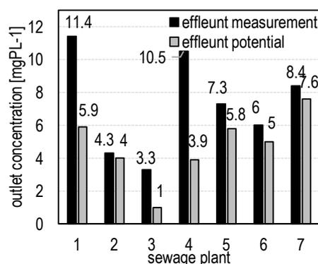
**Figure 9.** Optimization potential of selected activated sludge systems
