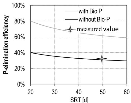
**Figure 5.** P-elimination efficiency in dependence of SRT of one selected WWTP
