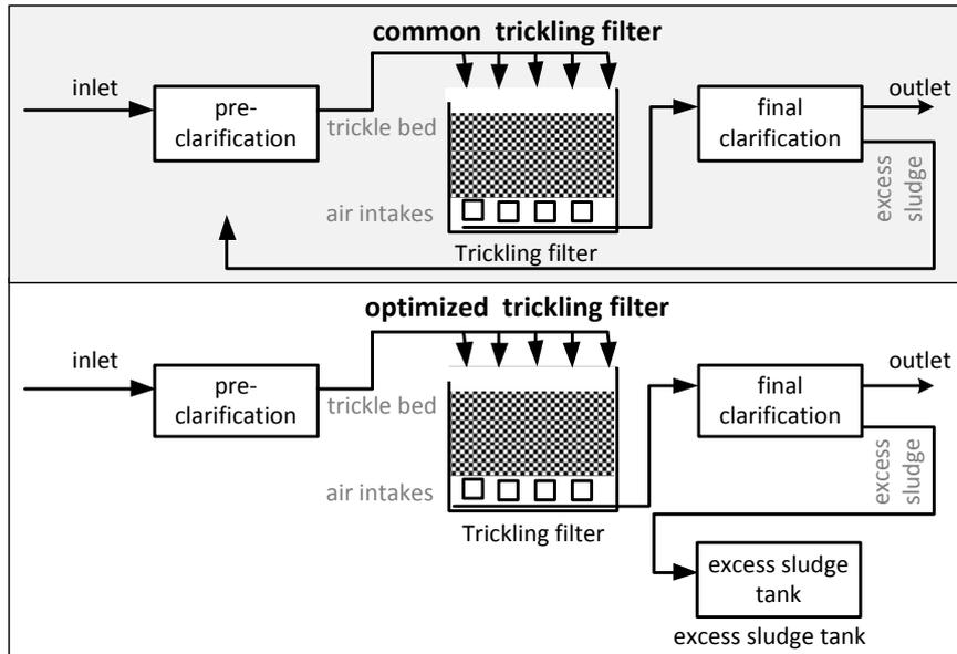
**Figure 7.** Schematic treatment technology of trickling filter
