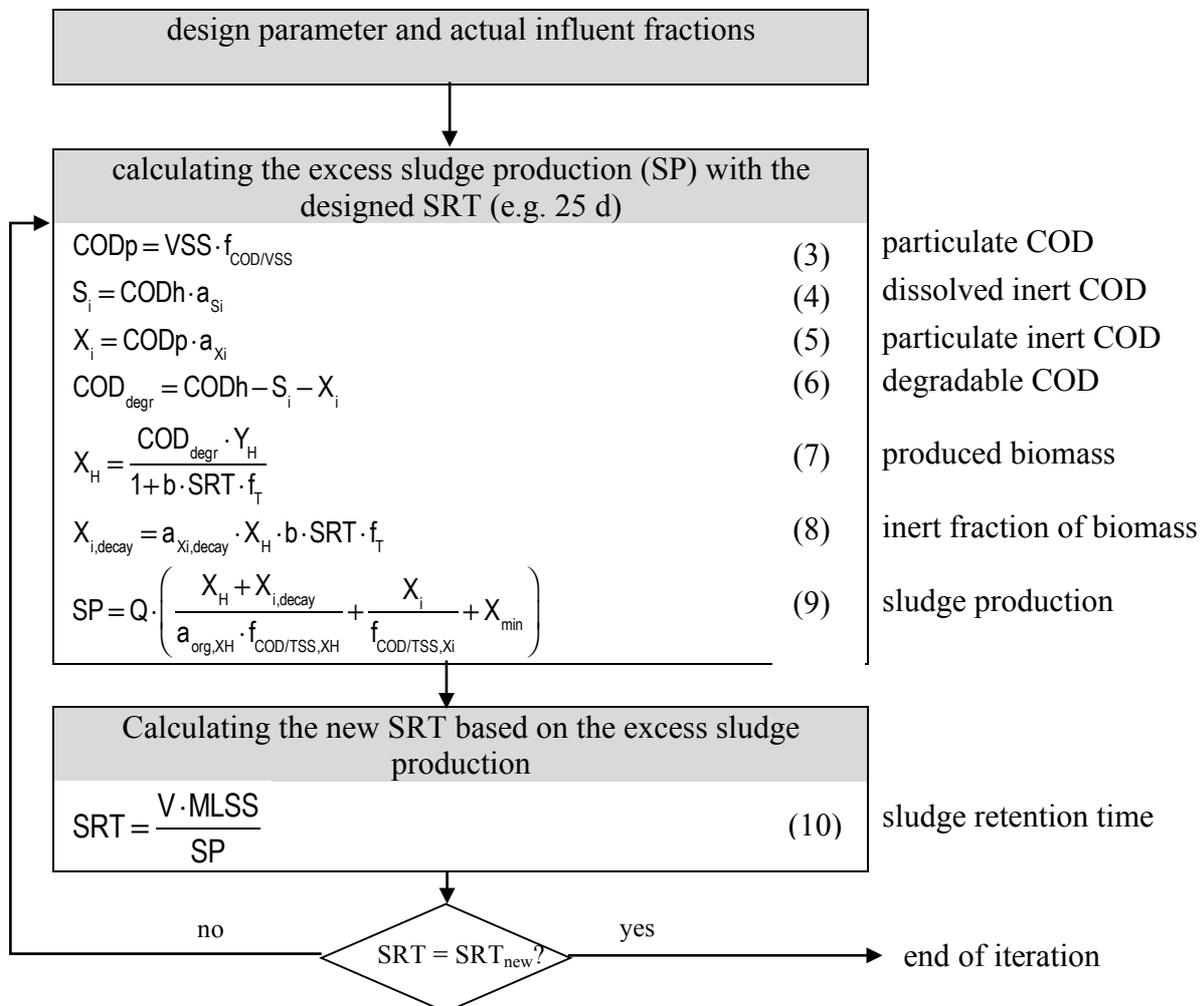
**Figure 1.** Iteration process for calculating the SRT by applying the COD approach
