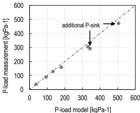
**Figure 4.** P-effluent-load for model verification based on 7 activated sludge systems
