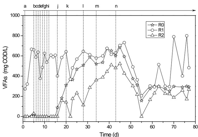
**Figure 4.** Effluent VFAs concentrations in system S0 (R0, control) and S1 (R1, R2) during the entire operational period.
