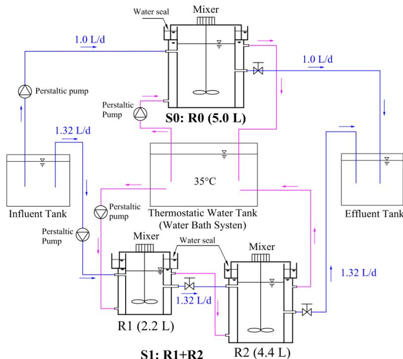
**Figure 1.** Schematic diagram of the one-stage (S0) and two-stage (S1) anaerobic systems.
