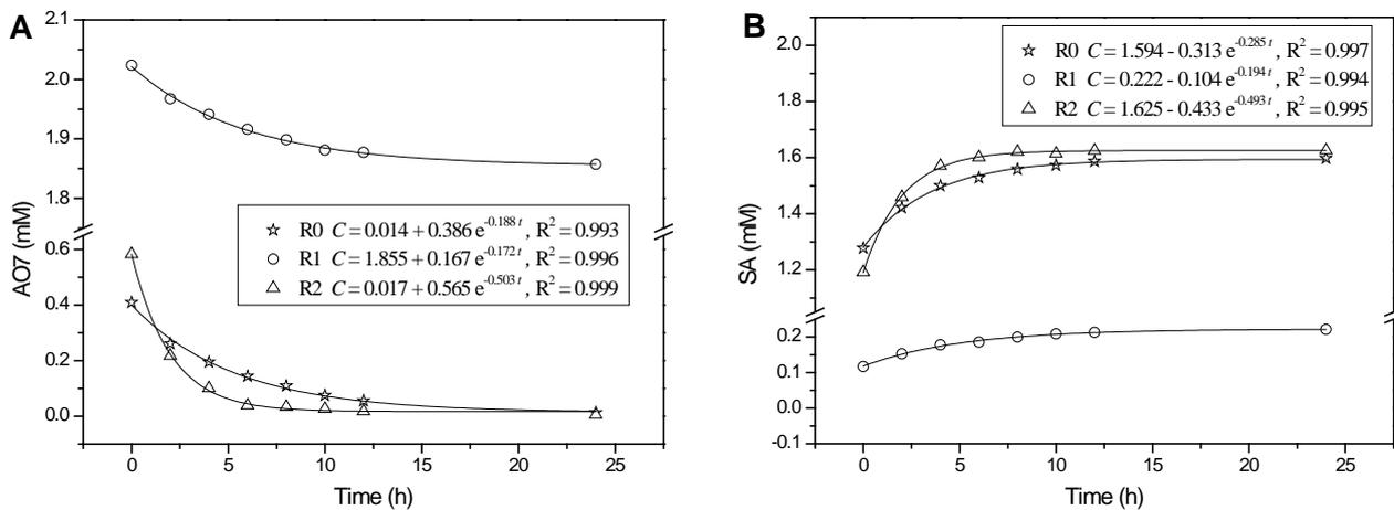
**Figure 3.** AO7 (A) and SA (B) concentrations at different time, and first-order kinetic fitting curves in one batch cycle of one-stage system S0 (R0, control) and one-stage system S1 (R1, R2).
