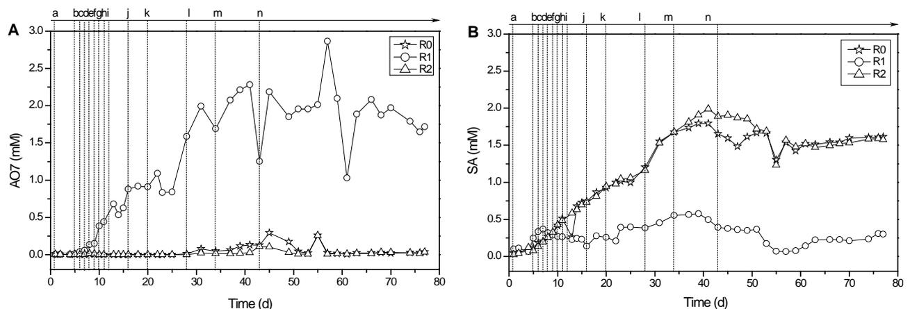
**Figure 2.** Effluent concentrations of AO7 (A) and SA (B) in system S1 (R0) and S2 (R1 + R2) during the entire operational period.
