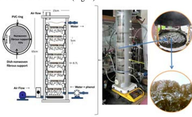
**Figure 1** Schematic diagram of the non woven flat plate bioreactor
