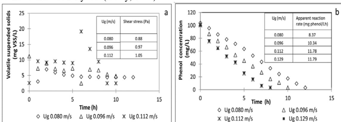
**Figure 4** a) Biofilm detachment in the reactor at different aeration rate ( $U_g$ ) values, b) Apparent reaction rate at different aeration rate ( $U_g$ ) values.
