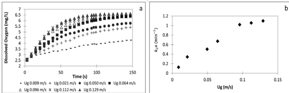
**Figure 3** a) Dissolved oxygen measurements at different aeration rate ( $U_g$ ) values, b) Values of the volumetric oxygen mass transfer coefficients ( $k_{L,a}$ ) considering different aeration rate ( $U_g$ ) values.
