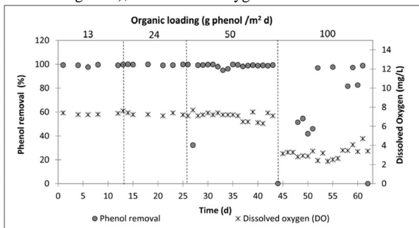
**Figure 6** Dissolved oxygen and phenol removal in a continuous reactor.
