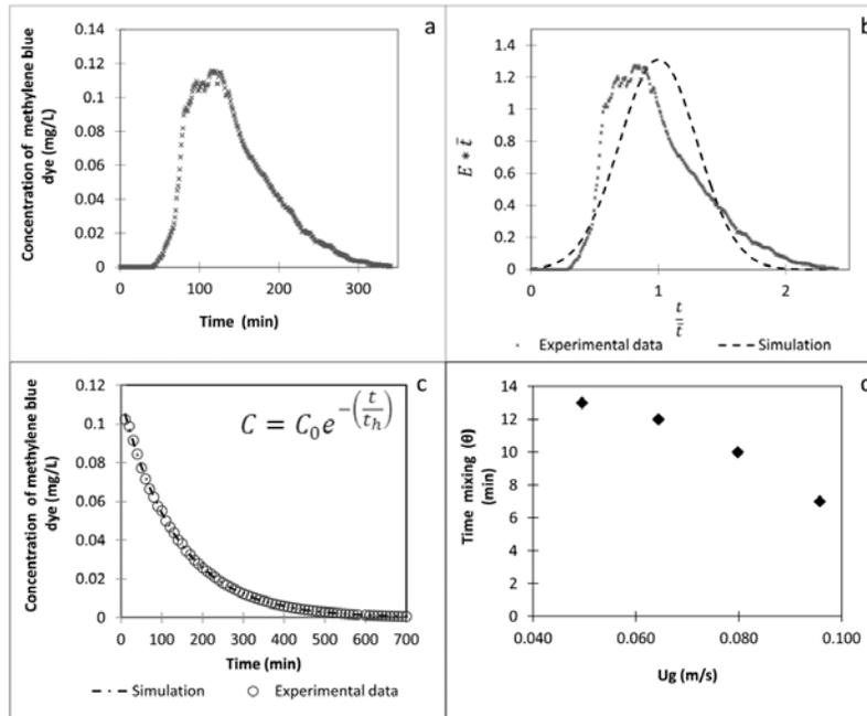
**Figure 2** a) Determination of the *RTD* curve without airflow, b) Modeling the *RTD* curve without airflow, c) Determination of the *RTD* curve with airflow, d) Measurement of the mixing time ( $\theta$ ) in the biological reactor at different aeration rate ( $U_g$ ) values.
