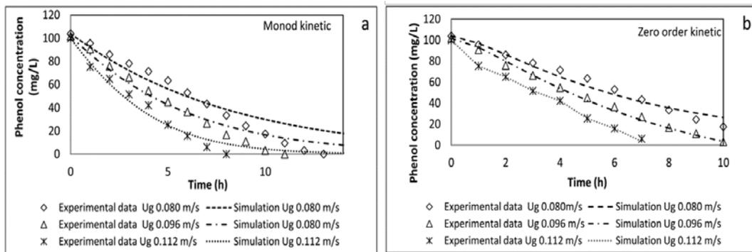
**Figure 5** a) Modeling at different aeration rate ( $U_g$ ) values with the Monod kinetic, b) Modeling at different aeration rate ( $U_g$ ) values with the zero-order kinetic.
