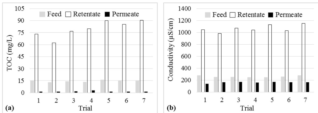
**Figure 5.** Rejection of TOC and TDS during 7 consecutive trials (water recovery = 88%)
