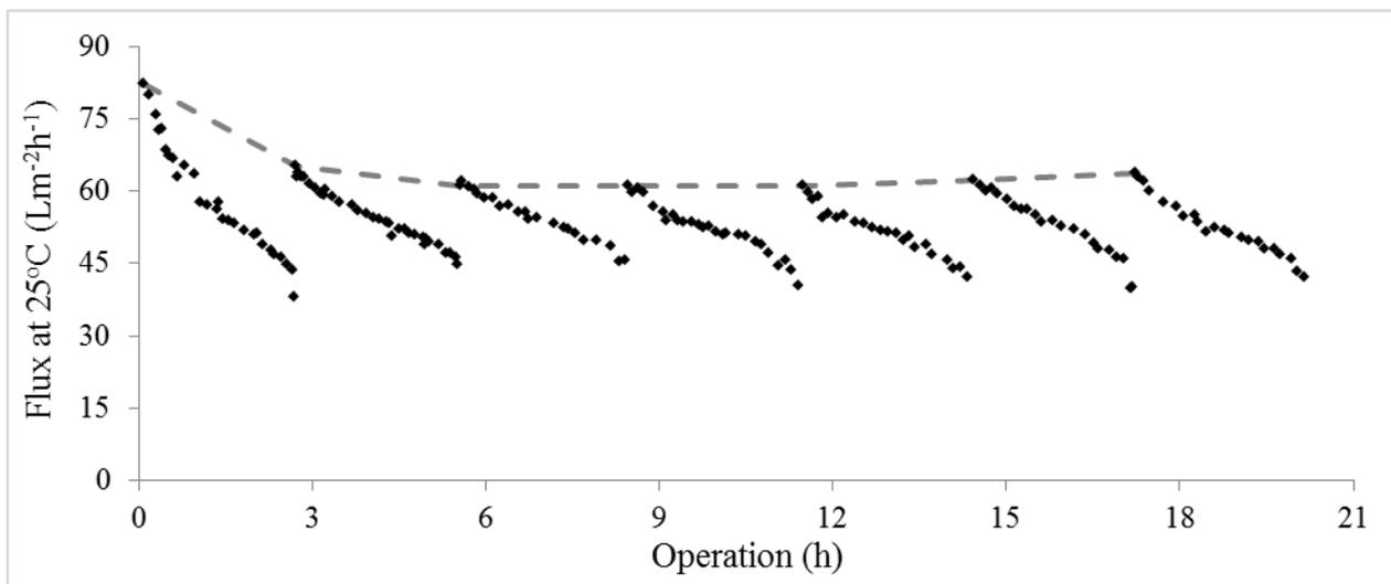
**Figure 3.** Change of permeate flux during nanofiltration cycles (WCF $\approx$ 0.88) – 7 operation cycles without membrane cleaning
