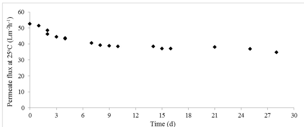
**Figure 6.** Decline in permeate flux during the fouling experiment at 5 bar
