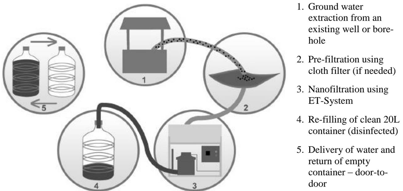
**Figure 7.** A sketch of operations in a micro-enterprise in a rural area [ from Ahmad (2015) ]
