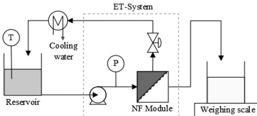
**Figure 2.** Schematic of the nanofiltration setup used in the study
