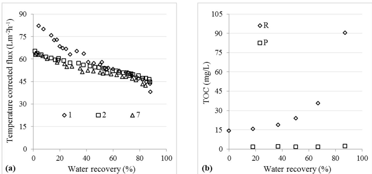
**Figure 4.** (a) Comparison of permeate flux from 1<sup>st</sup>, 2<sup>nd</sup> and 7<sup>th</sup> trials; (b) TOC content in retentate (R) and permeate (P) during concentration of model ground water – from trial 7
