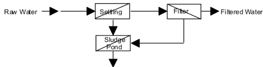
**Figure 1a. Treatment Plant with No Sludge Lagoon Supernatant return**
