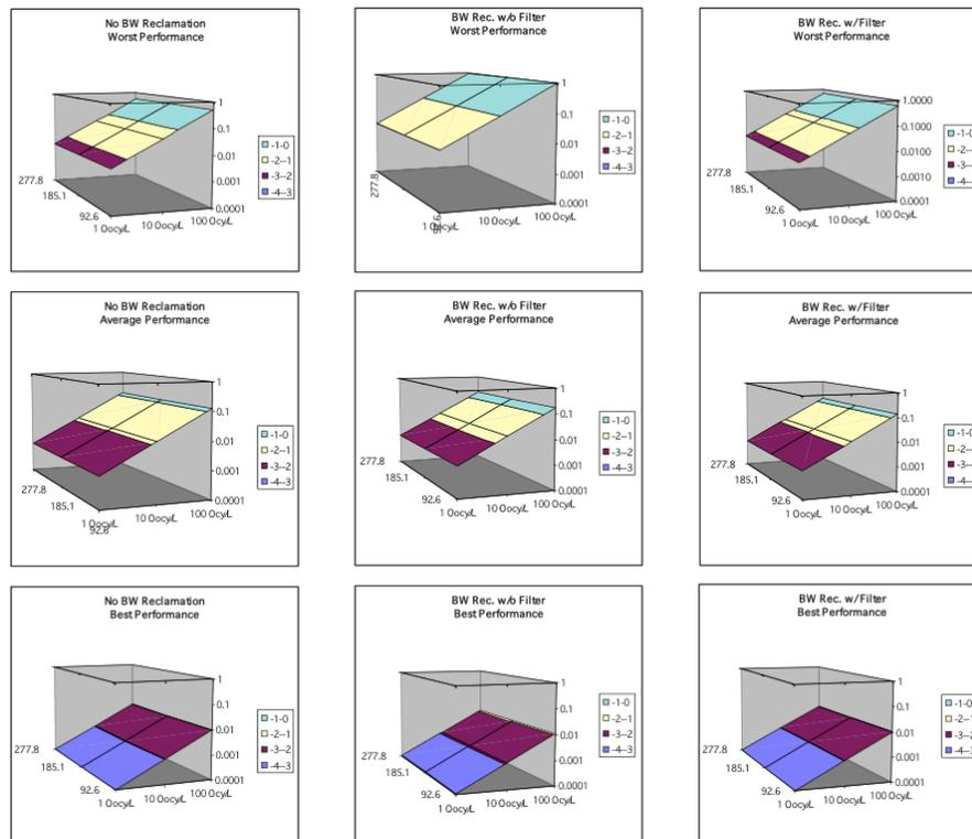
Figure 2. Treatment plant *Cryptosporidium* oocyst removal performance based on plant flow
