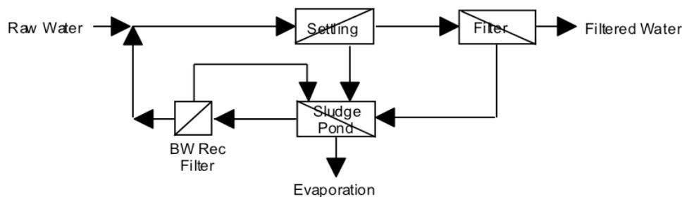
**Figure 1c. Treatment Plant with Sludge Supernatant return, With Filtration**
