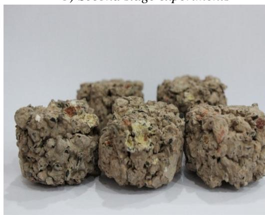
d) Porous media prepared by laterite soil and other composites
