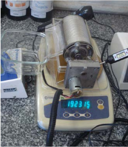
Figure 3: Experimental set up: the urine evaporating reactor and collection of the precipitate.
