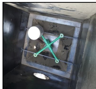
(c) A module of cartridges installed at the bottom of a compartment in the fabric filter unit
