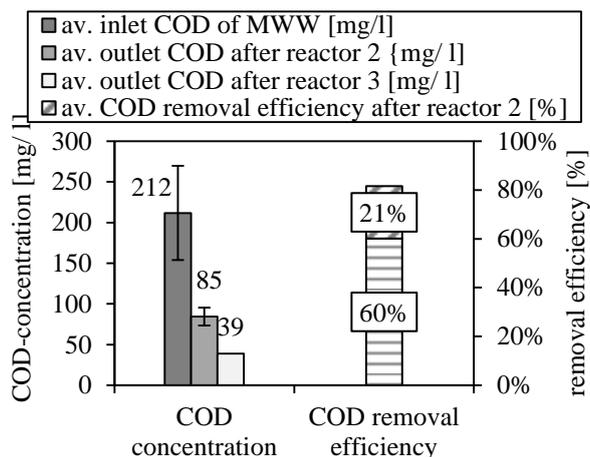
**Figure 6:** Average organic degradation performance of the pilot plant treating municipal wastewater (MWW) within 200 days of operation. The average COD concentrations for the incoming MWW, for the outlet of R2 after the anaerobic digestion and for the outlet of R3 after the Anammox-based process are plotted. Furthermore the COD removal efficiency for the anaerobic digestion as well as for the Anammox-based process are shown.
