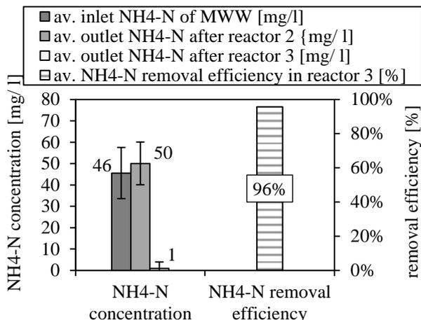
**Figure 7:** Average ammonium degradation performance of the pilot plant treating municipal wastewater (MWW) within 200 days of operation. The average NH<sub>4</sub>-N concentrations for the incoming MWW, for the outlet of R2 after the anaerobic digestion and for the outlet of R3 after the Anammox-based process are plotted. Furthermore the NH<sub>4</sub>-N removal efficiency for the anaerobic digestion as well as for the Anammox-based process are shown.
