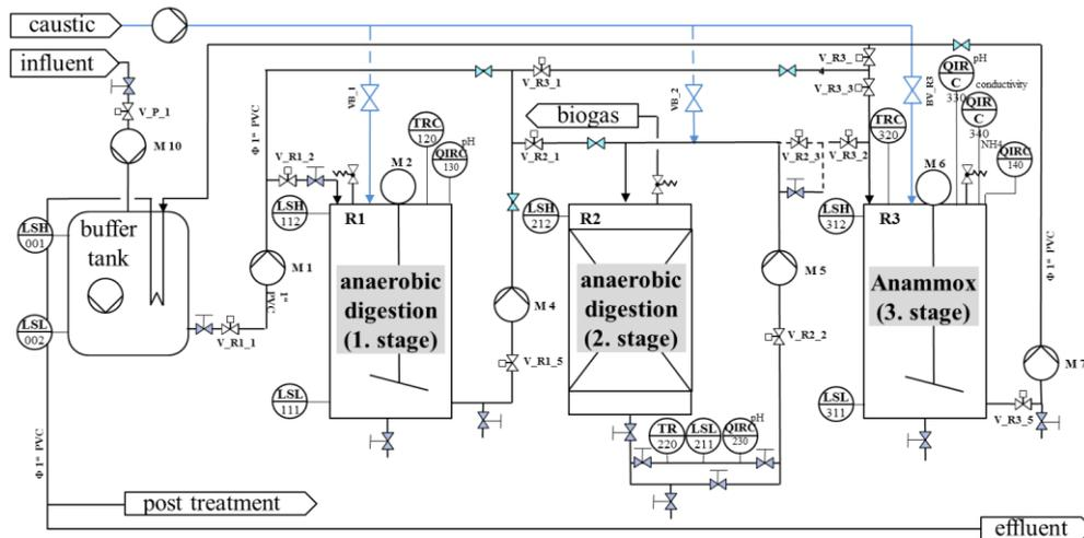
**Figure 2:** Process and instrumentation scheme of the decentralised anaerobic pilot plant for producing domestic service water out of domestic wastewater.
