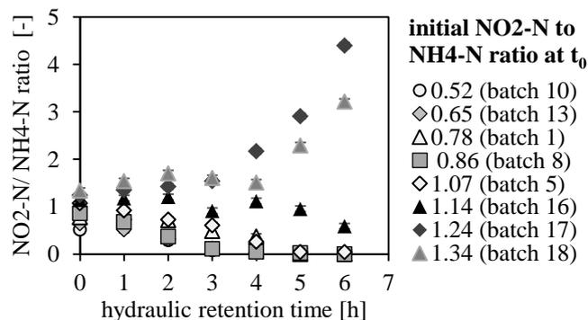
**Figure 5:** Determination of optimal initial substrate to feed ratio of NO<sub>2</sub>-N to NH<sub>4</sub>-N over 6 hours retention time during the Anammox process treating municipal wastewater.
