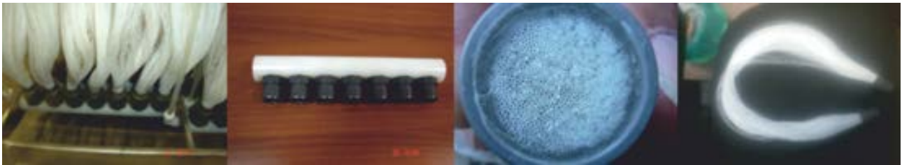
Fig.4. GOST submerged hollow fibre membrane module and bundle (courtesy of GOST MBR solutions).
