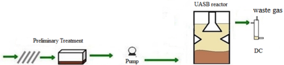
Figure 1: Schematic configuration of experimental apparatus.
