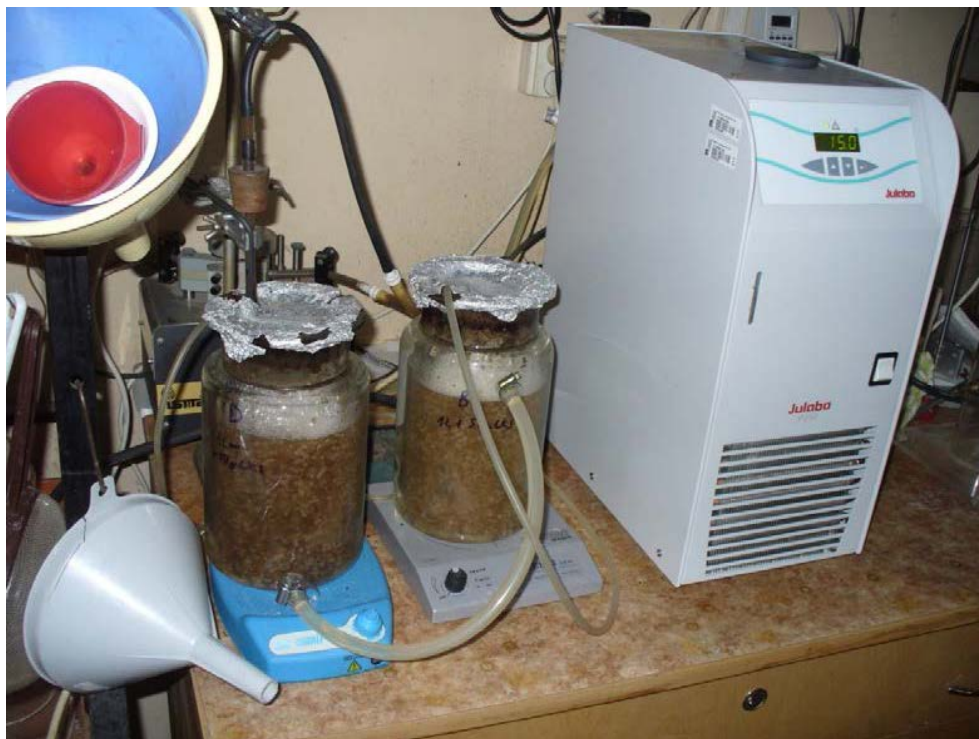
Figure 2. Reactors used for experiments of nitration inhibition with hydroxylamine
