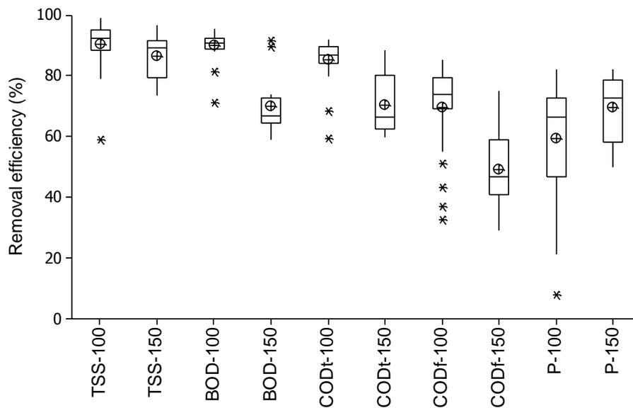
**Figure 3:** Removal efficiency for TSS, BOD, homogenized COD (COD<sub>t</sub>), filtrated COD (COD<sub>f</sub>) and total phosphorous (P) of a greywater treatment plant at 100% and 150% nominal load (25;50:75 percent quartiles in the box plots with 95% quartiles in the error bars; average is indicated in the point plot)
