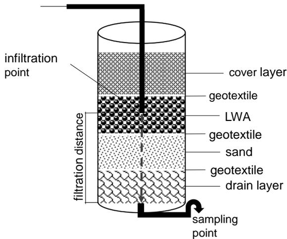
**Figure 1.** Cross section of an infiltration trench column consisting the following layers: 200mm of top soil (excavated at Aas, Norway); 150mm of lightweight aggregate LWA 2-4mm; 150mm of sand 0.2-1.0mm; 150mm of crushed stone 11-22 mm, giving a total filtration distance of 375mm.
