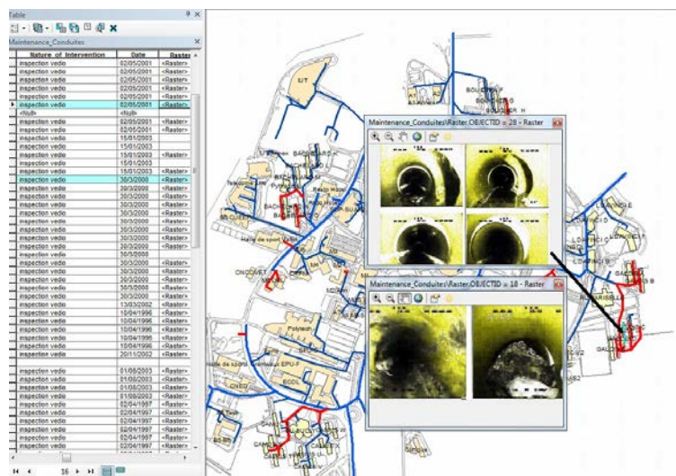
Figure 7: The inspection layer and an example of a detected system structural failure
