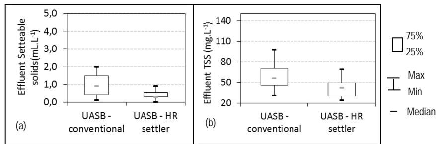
**Figure 2.** Effluent settleable solids (a) and effluent TSS (b) concentrations from the conventional UASB reactor and from the UASB reactor equipped with the high rate settler.
