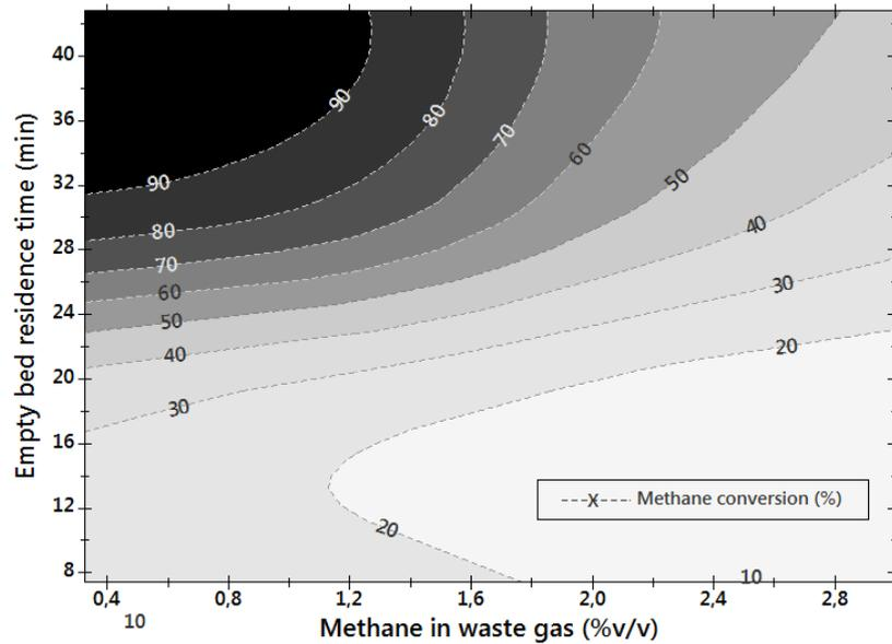
**Figure 3.** Contour plots showing the effect of the CH<sub>4</sub> in waste gas and the empty bed residence time on CH<sub>4</sub> abatement in biofilters packed with composted leaves (60%<sub>v/v</sub>) and expanded vermiculite (40%<sub>v/v</sub>).
