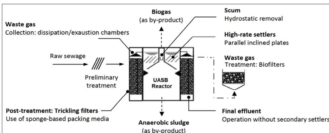
**Figure 1.** Compact UASB/SBTF system for sewage treatment in developing countries. The continuous lines indicate the proposed improvements for the technology.
