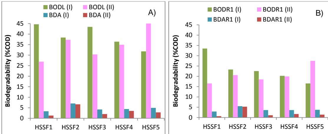
**Fig. 3.** Aerobic (BOD) and anaerobic (ABD) biodegradability of accumulated solids COD during campaigns I and II (A: total biodegradability obtained from  $BOD_L$  and final ABD values, B: readily biodegradability obtained from the initial R1 high rate period).
