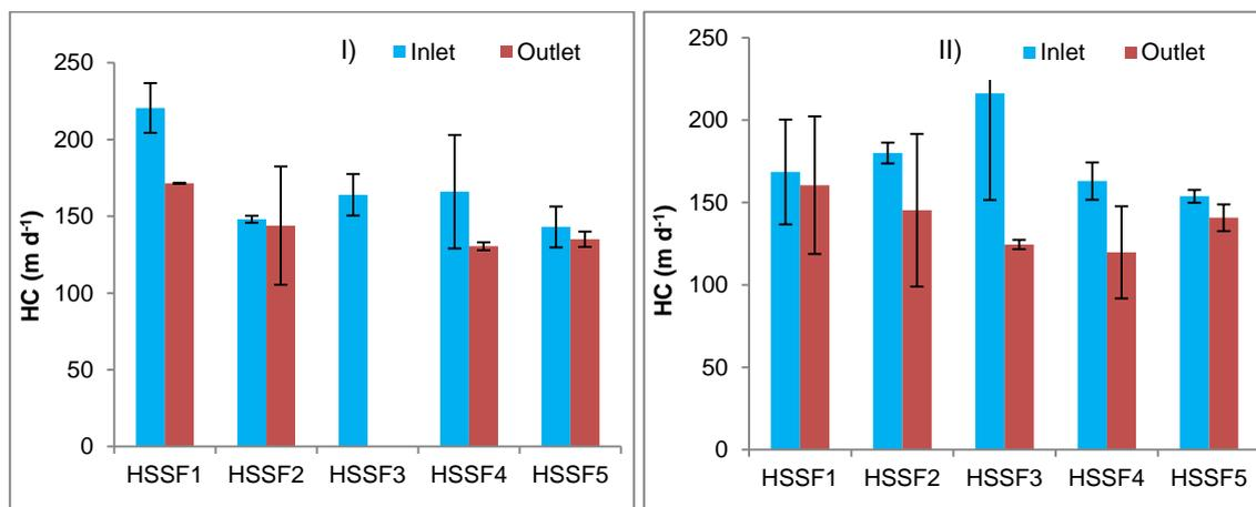
**Fig. 4.** Hydraulic conductivity of gravel medium at near the inlet and near the outlet zones during campaign I (left) and campaign II (right). Each bar corresponds to the mean value obtained for the same transversal position ( $n=4$ ) while error bars correspond to standard deviation.
