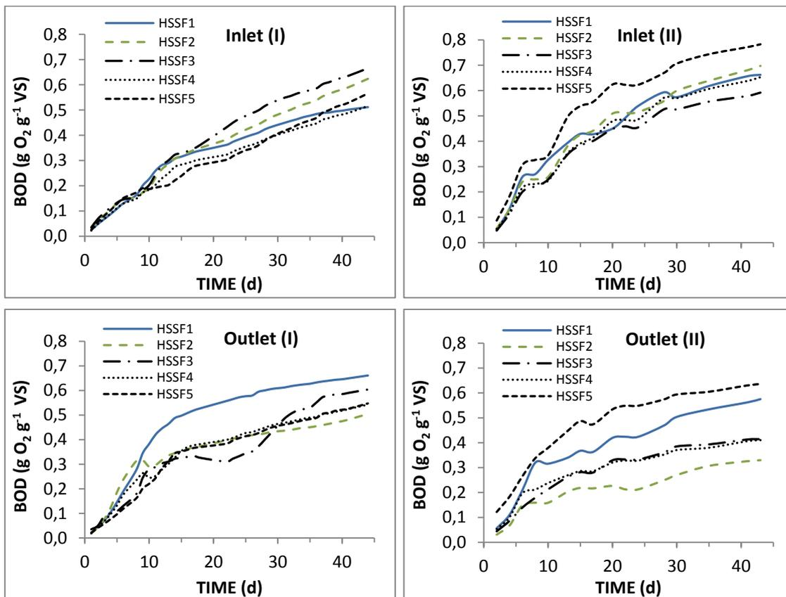
Fig. 1. Time profiles of aerobic biodegradability (BOD curves) of accumulated solids in HSSF units.
