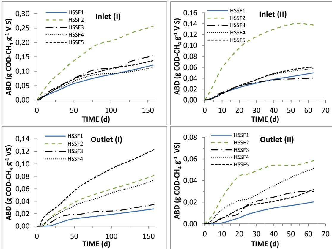
**Fig. 2.** Time profiles of anaerobic biodegradability (ABD curves) of solids from near the inlet and near the outlet of HSSF units at campaigns I and II.
