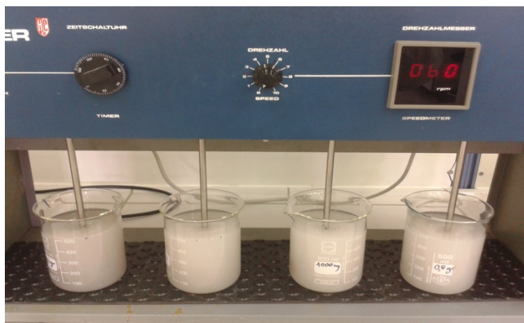
Figure 1. Jar test apparatus.
