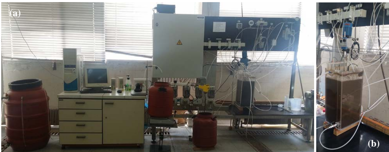
Figure 1. (a) Pilot-scale MBR system, (b) aeration tank (bioreactor).
