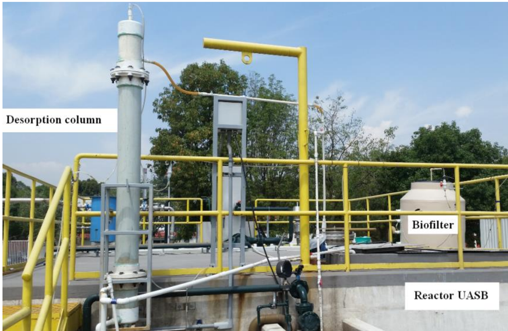
Pilot system for the biological removal of dissolved \text{CH}_4 in a UASB effluent
