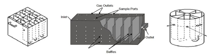
In the ABR the liquid flows downward and upward through the chambers
