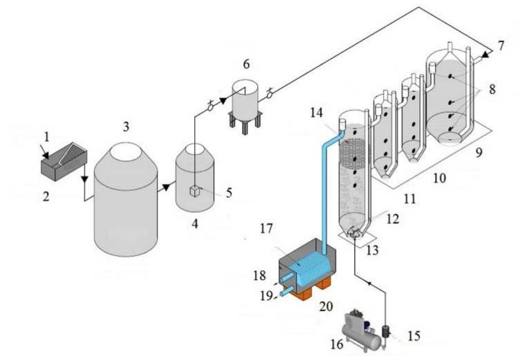
**Figure 1**. Schematic diagram of the AABR: 1-Wastewater; 2- Screen; 3- Settling tank; 4-Equalization tank; 5- Pump; 6- Storage tank; 7- Influent; 8- Chambers sampling points (for the present study, the higher points were used); 9- Chamber 1; 10-Chamber 2; 11- Chamber 3; 12-Air diffusers; 13- Aerobic chamber; 14- Bamboo rings; 15- Air flow meter; 16- Air compressor;
