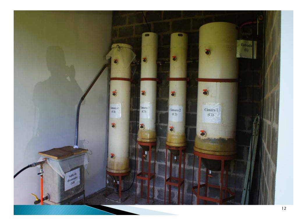
Anaerobic/aerobic Baffled Reactor (AABR)
