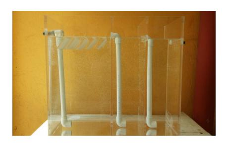
A lab-scale UASB-septic tank (45 L volume, acrylic), consisting of three compartments treated high strength municipal wastewater from the Metropolitan Autonomous University - Azcapotzalco Campus.
