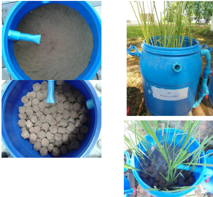
0.65 cm porous media+ 5 cm sand 0.8 m height and 0.45 m dia.
