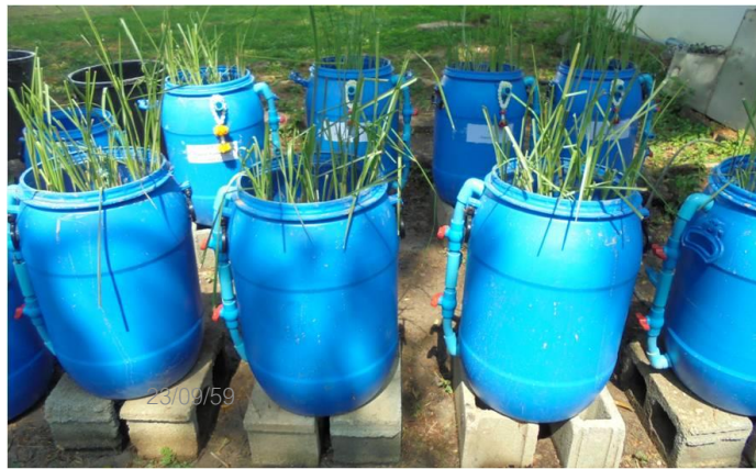
0.65 cm porous media+ 5 cm sand 0.8 m height and 0.45 m dia.
