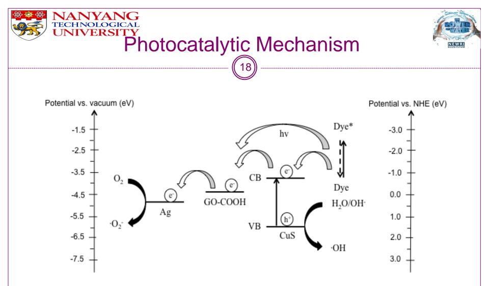
Schematic illustration of proposed electron transfer mechanism of GO-COOH-CuS-Ag nanocomposites.
