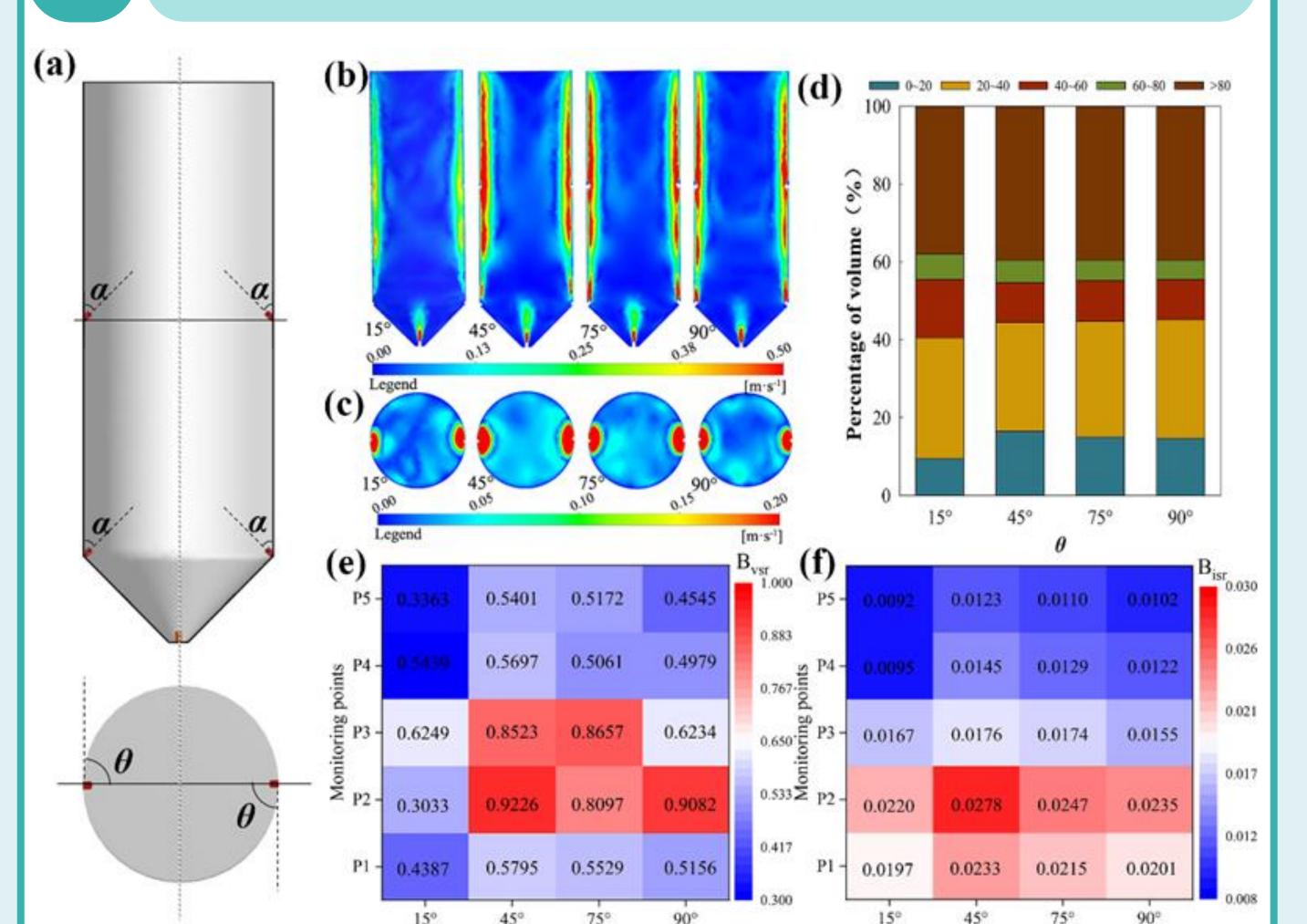
The reactor exhibited a working volume of 20 L, with a conical height of 90 mm, cylindrical height of 500 mm (H=590 mm, D=200 mm).
