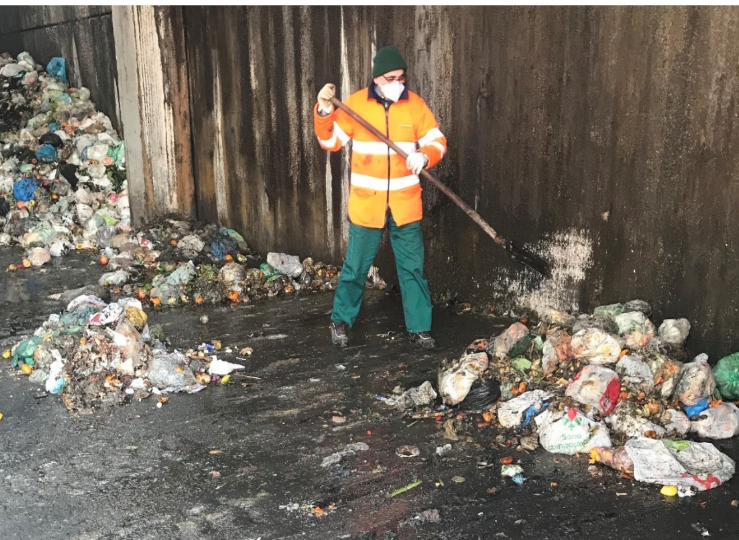
Figure 1. Quartering method procedure
