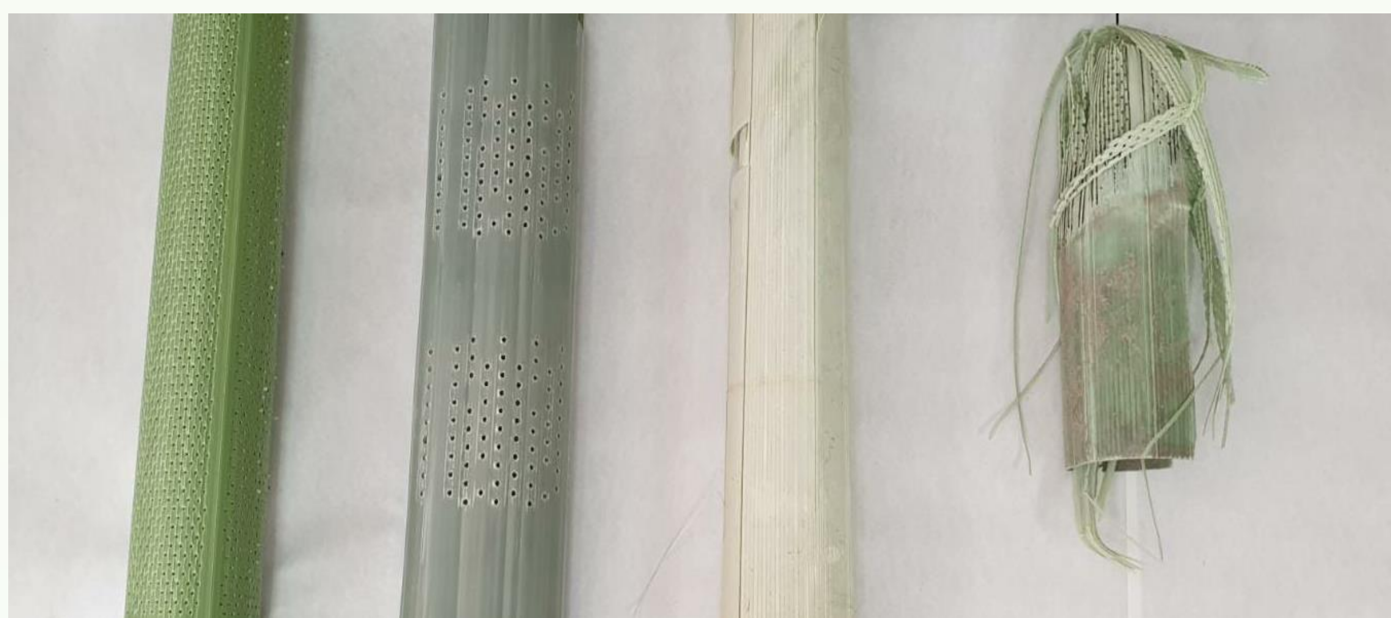
Fig 1. From left to right: new, 5 years, 10 years and 20 years old tube shelters
