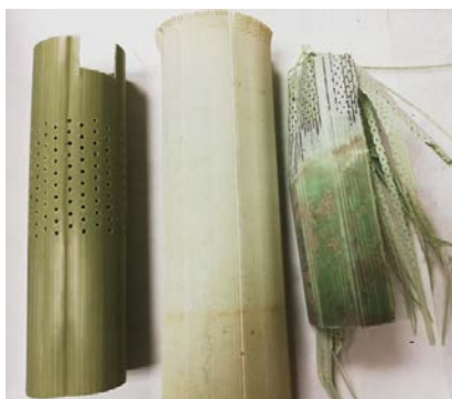
Fig. 1. PP tree shelters not used (left) and recovered from different reforestation processes carried out in Spain, 10 and 20 (right) years ago.
