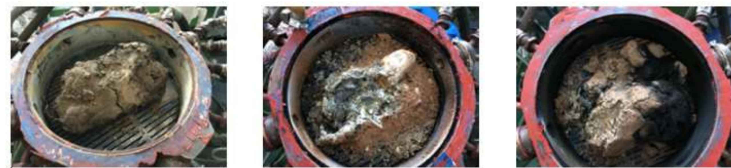
Fig. 2 Bituminous soil before treatment (a) and after treatment with water vapor plasma (b) or air plasma (c)
