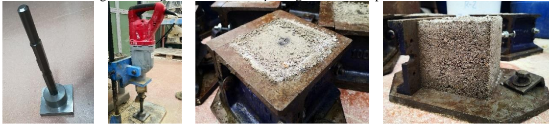
Figure 1. Images from vibro-compacting method and specimens casted.
