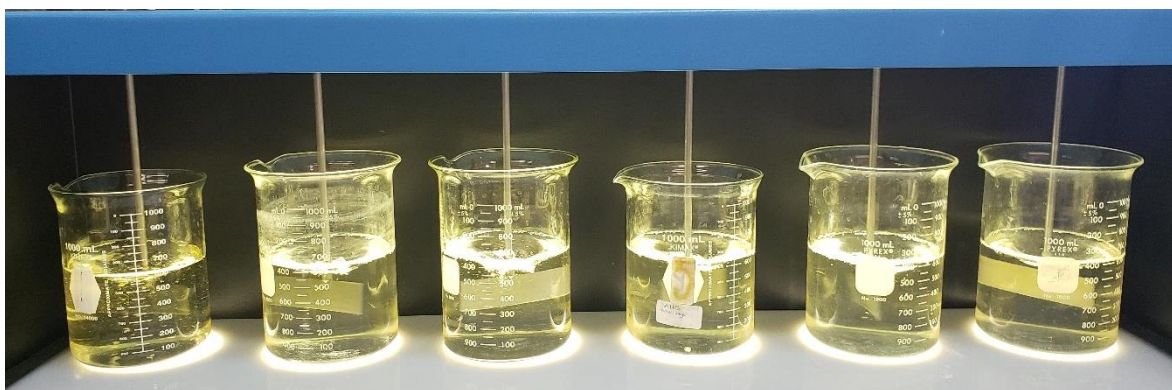
Figure 3. Jar testing in the Sanitary and Environmental Engineering Laboratory.
