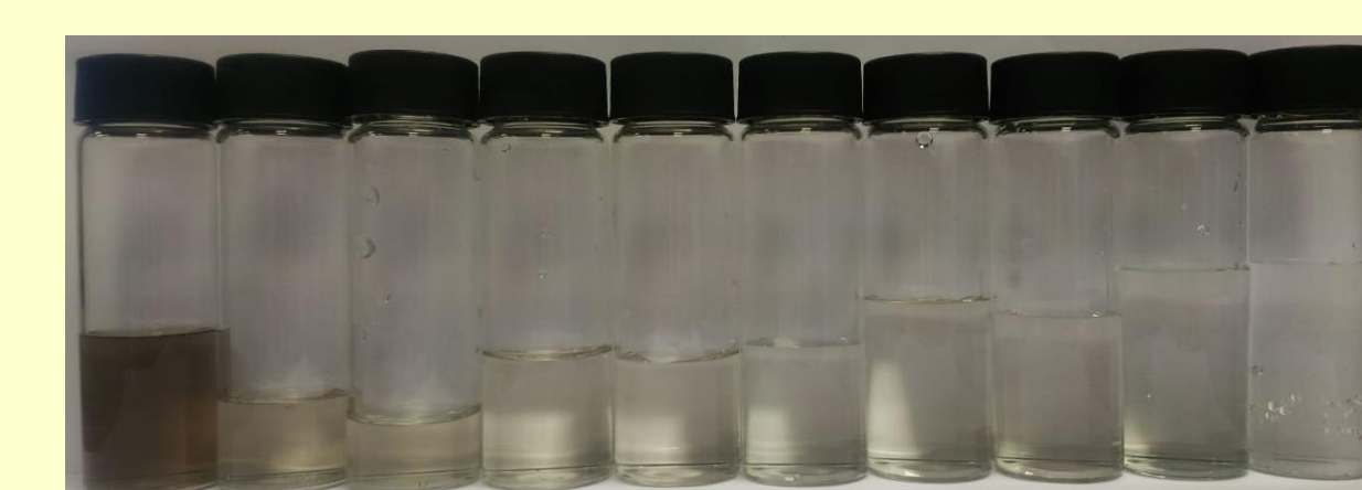
Figure 5 : Real Textile wastewater aliquots during adsorption kinetics by biochar at pH 6, room temperature
