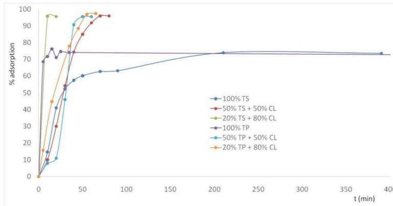
**Fig. 1** Percentage of methylene blue adsorption from its aqueous solutions on different mixtures of tangerine by-products and zeolites activated with HCL acid (4M) versus time, t, at a ratio of 10 g adsorbent L<sup>-1</sup> adsorbate
