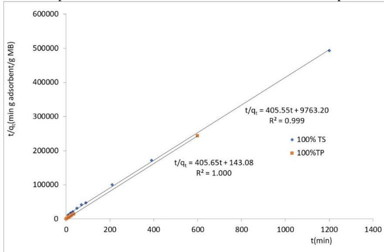
**Fig.4** Application of pseudo-second order kinetic model to the experimental adsorption data of methylene blue dye (MB) on chemically modified tangerine peels (TP) and tangerine stones (TS).
