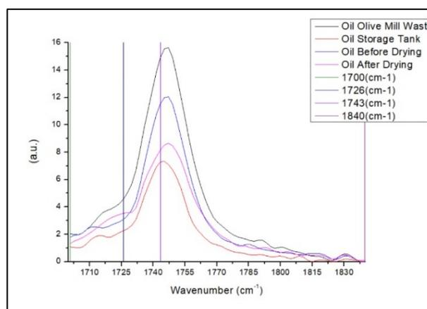
Fig. 3. FT-IR analysis of the examined samples
