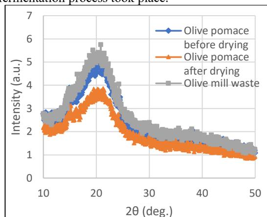
Fig. 2. XRD analysis of the examined samples
